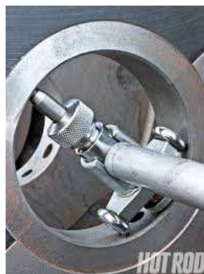
Fig.22 Using bore gauge showing measuring sled
