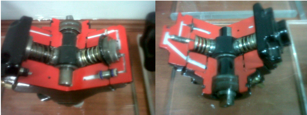
Fig 16 : Cut section view of high pressure pump
