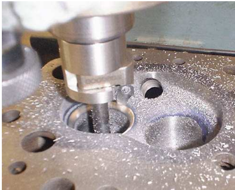
Fig 9 : Seat Cutting operation
