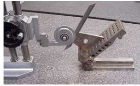
Using a protractor with a vernier height gauge
