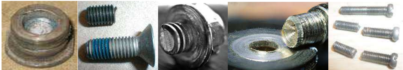
Fig- 24 Broken and spoiled screw
