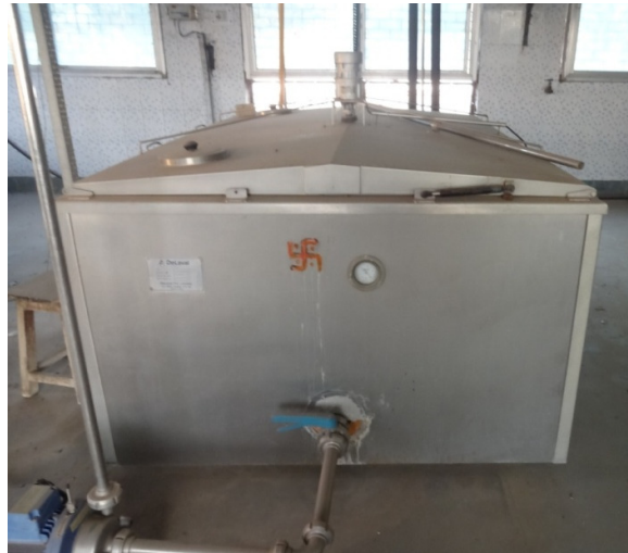
Figure 2.7: Milk chilling tank of 1000 litres capacity
